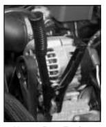
The remote negative (–) terminal is located on the engine accessory drive bracket and is marked "GND" for all Vortec 5300 engines. It is located on the thermostat housing and marked "GND" for all Vortec 8100 engines.
